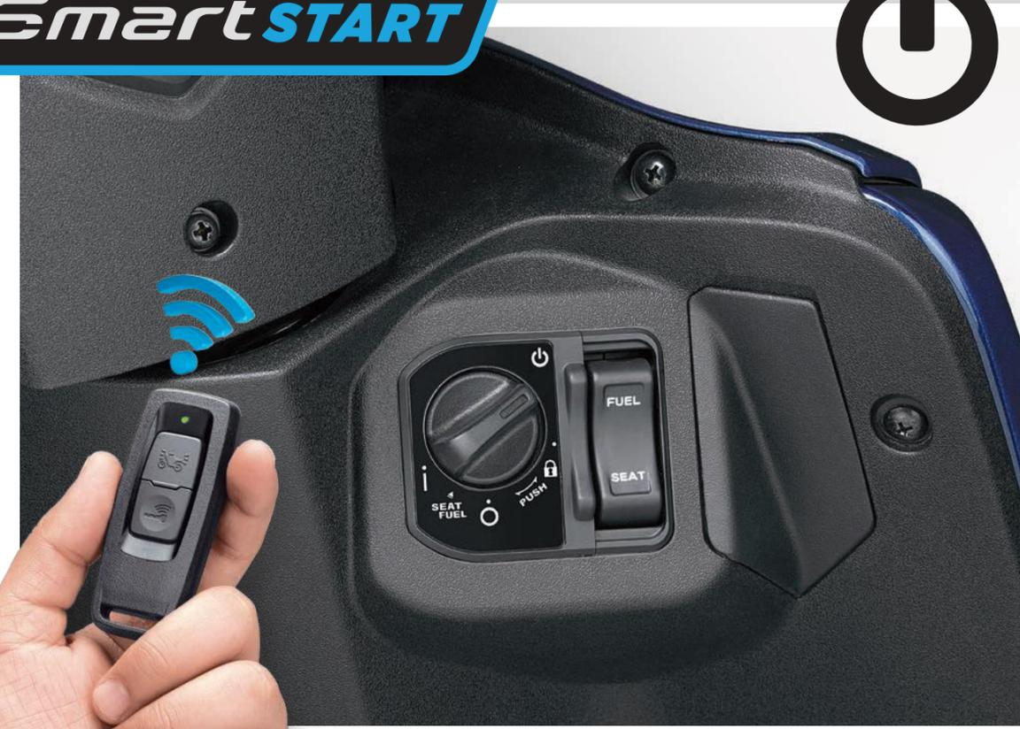
Here's a way to start your ride that doesn't even require you to take out the key from your pocket! Once the key is within **2 meters** of your Activa, and activated, all you have to do is **push the knob** – the LED Smart Key indicator on the speedometer will come on – then just rotate the knob to **turn on the ignition and start the engine with Start/Stop switch.**
